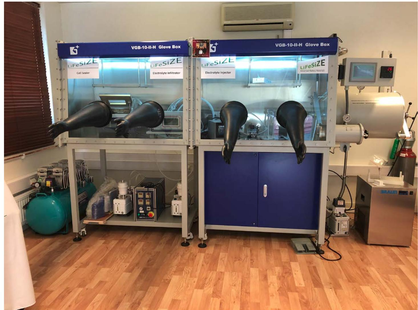
**Cells on their way into the heatable, evacuable glovebox ante-chamber (typical treatment: overnight at 75°C)**
