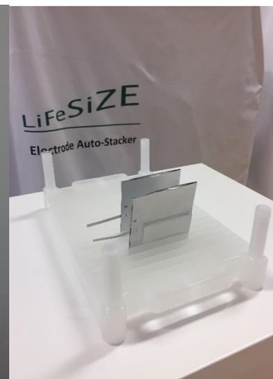
**Cells placed in a glovebox rack-sealed along three sides prior to electrolyte injection**
