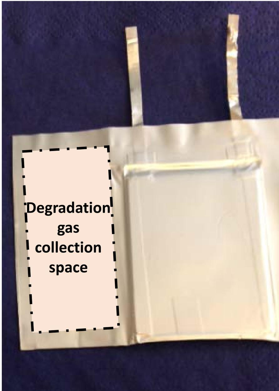
**A Li-/Na-ion battery-cell prototype –
